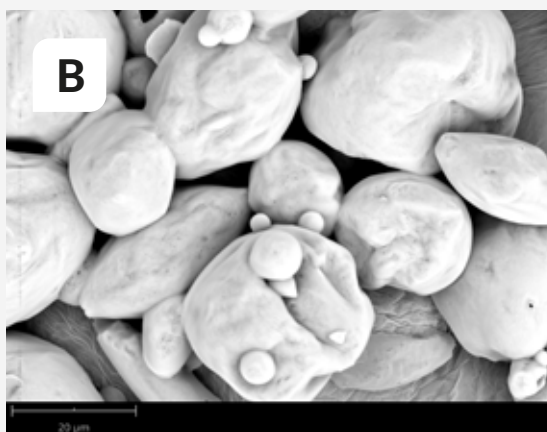
Fig. 3. Liposovit®-Glutathione powder particles in images obtained under the scanning electron microscope (Phenom XL, Phenom World BV). A. Magnification of 1000 x, B. Magnification of 3000 x.
